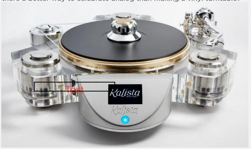
As often, the technology is not visible: the device stability is assured by 3 adjustable feet with magnetic fluid suspension, and the platter itself is floating on magnets. The separate motor speed is electronically controlled and the tonearm fully adjustable (vertical angle, azimuth, anti-skating) with 3 counterweights to adapt to all cartridges up to 21 grams.
